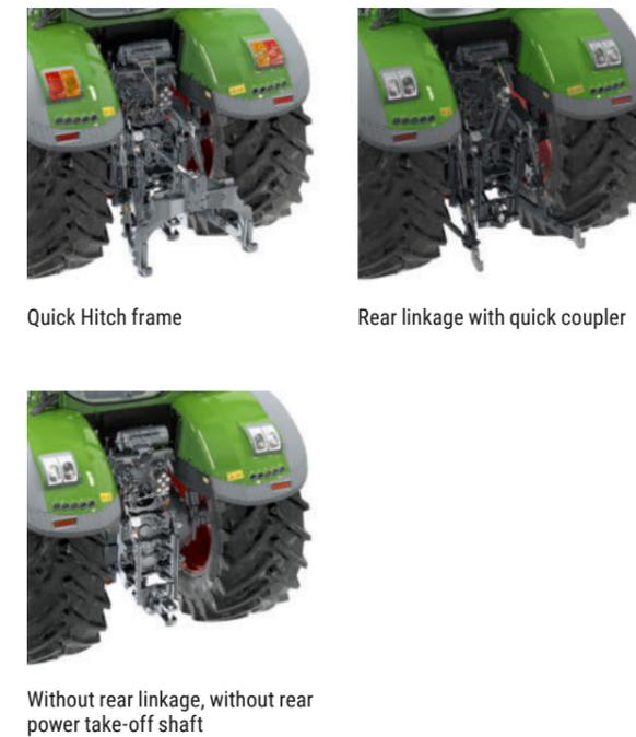
Quick Hitch frame      Rear linkage with quick coupler
